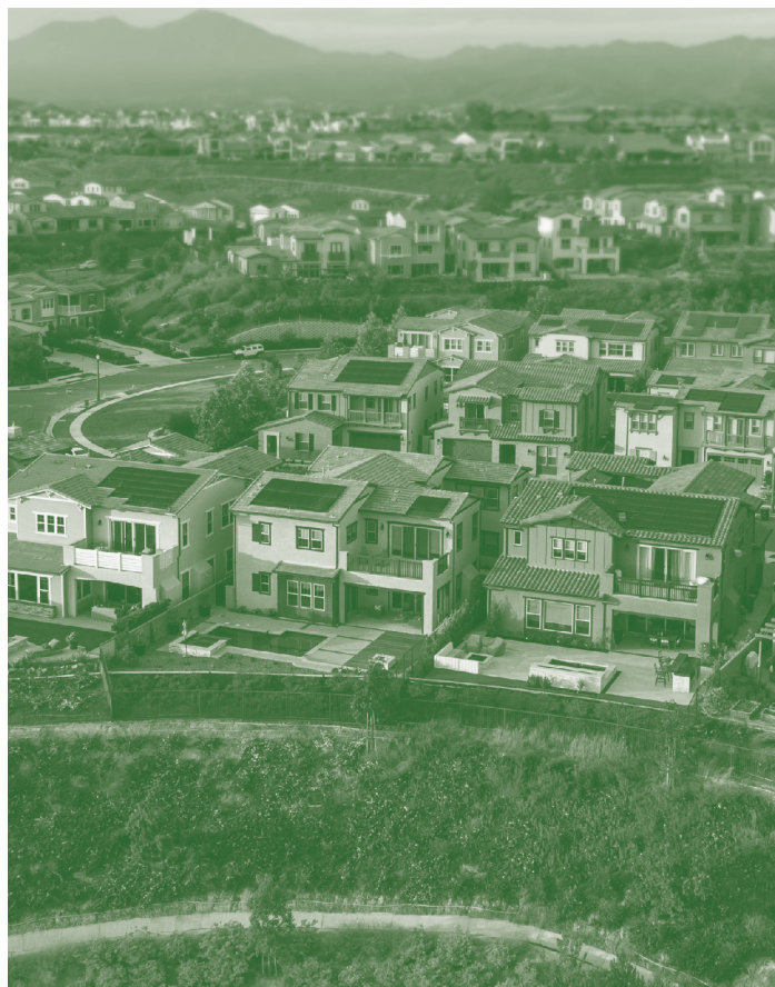
Subdivision in Orange County with houses surrounded by fuel modification zones. Image: Jonnu Singleton, SWA
